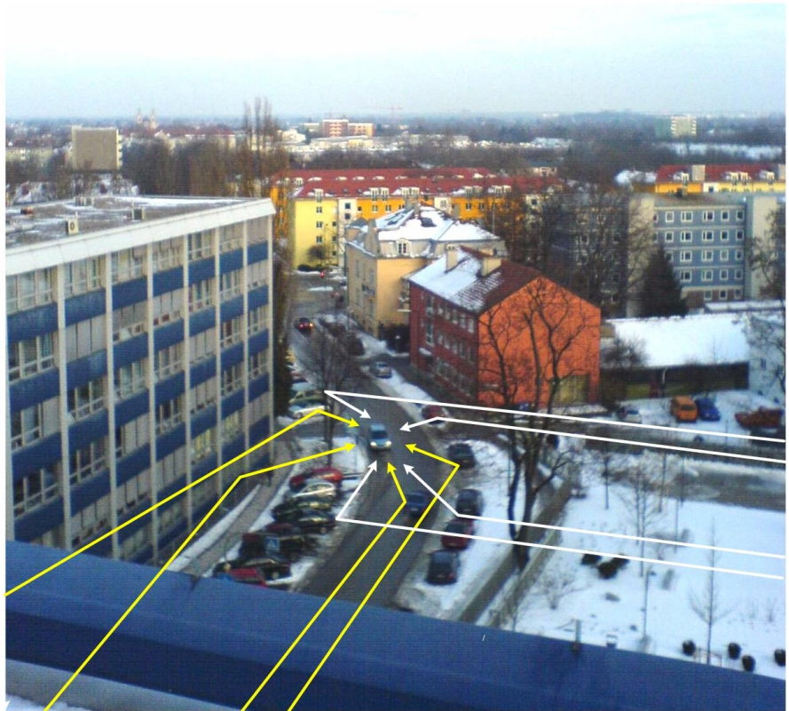
Fig. 5_1: Typical multipath condition in the city for a mobile radio installed in a car.
